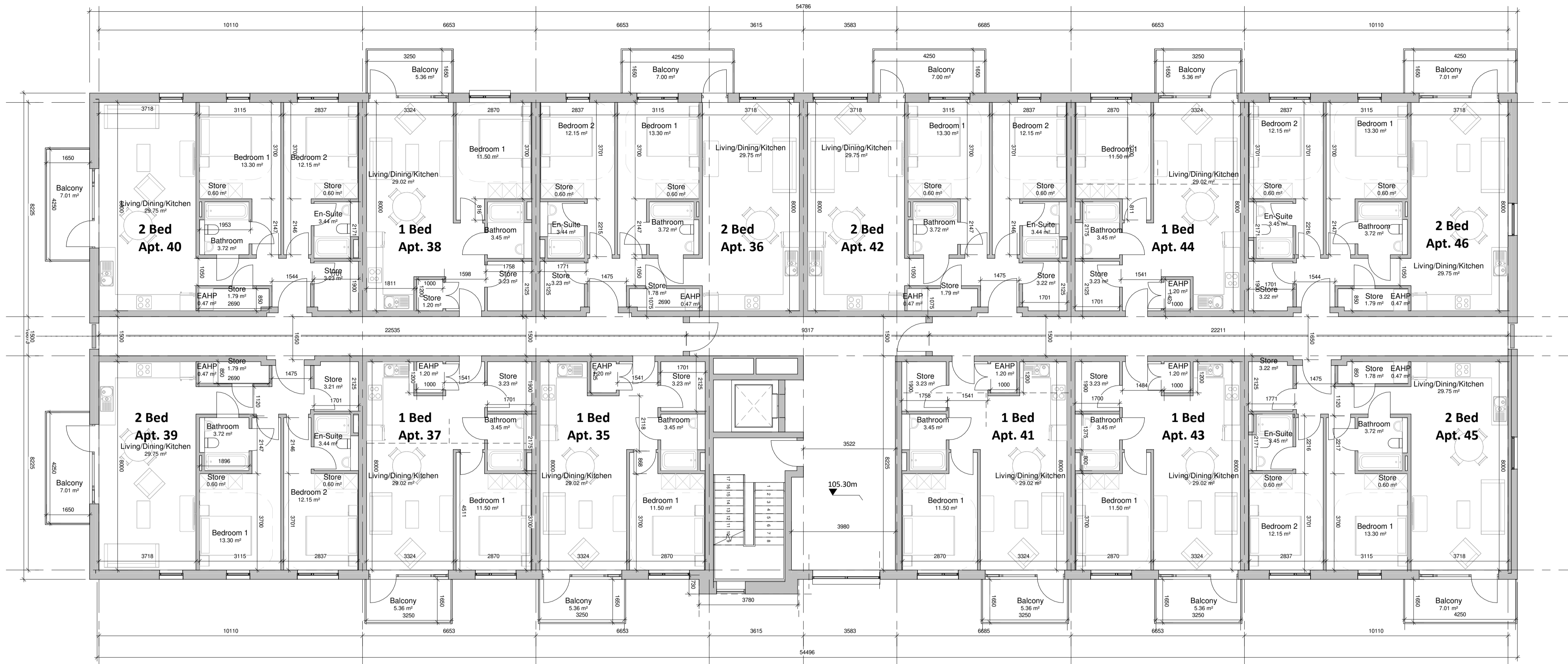
1 THIRD FLOOR LEVEL - BLOCK B 1 : 100
